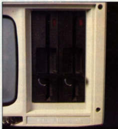
Top: The Miracle's 386K disk drives. Below: External controls are for brightness and on/off
